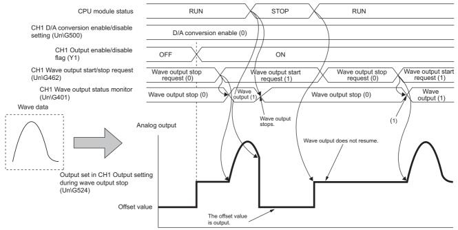
(1): Wave output starts when the value set in CH1 Wave output start/stop request (Un\G462) is changed from Wave output stop request (0) to Wave output start request (1).
