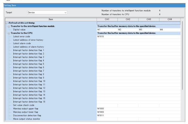
**8.** Write the set parameters to the remote head module on the intelligent device station. Then reset the remote head module or power off and on the system.
