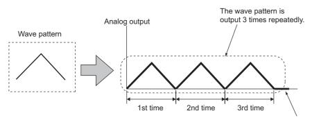
After the wave pattern is output 3 times, wave output stops and an analog value is output according to the setting in CH1 Output setting during wave output stop (UnG\524).
