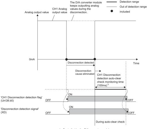
· - - Controlled by the D/A converter module
