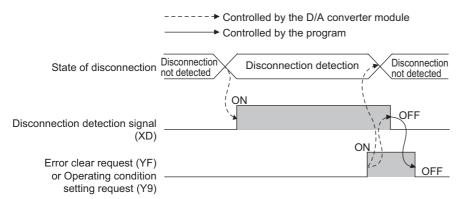
When 'CH1 Disconnection detection auto-clear enable/disable setting' (Un\G561) is Enable (1), however, if any other disconnections have not occurred until CH1 Disconnection detection auto-clear check monitoring time<sup>\*1</sup> elapses, 'Disconnection detection signal' (XD) automatically turns off.
