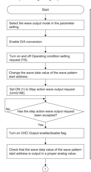
Example of testing analog output in CH1
