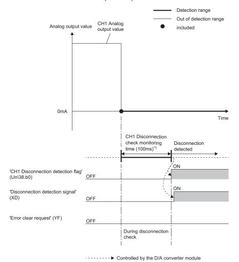
\*1 CH1 Disconnection check monitoring time is calculated with the following formula.
