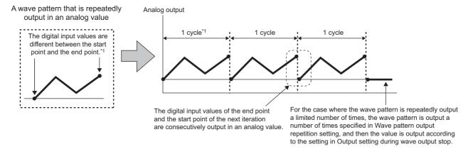
\*1 The output cycle of a wave pattern is calculated by the following formula.
