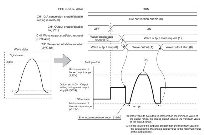
In addition, when the digital input value out of the range is set and an error (error code: 191 $\square$ H) has occurred, correct the value to the one within the range and turn on and off 'Error clear request' (YF).
