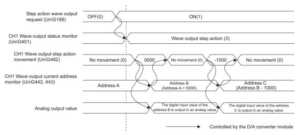
Change the value in 'Step action wave output request' (Un\G188) from OFF (0) to ON (1) to set the wave output status to the wave output step action. By setting a value in 'CH1 Wave output step action movement amount' (Un\G482) during the wave output step action, the address moves to the address of the target wave data for the output test. Set the amount for movement from the current wave data address in 'CH1 Wave output step action movement amount' (Un\G482).
