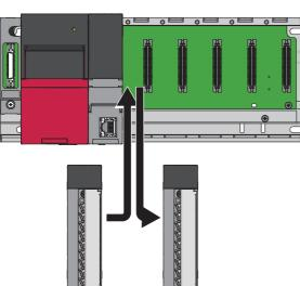
2. Replace the D/A converter module.
