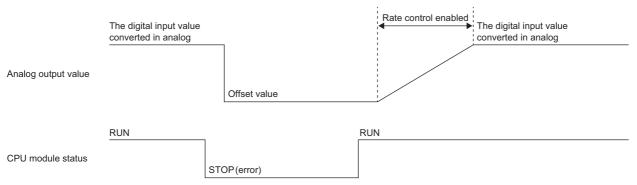
• When the CPU module status is changed from STOP (error) to RUN while the D/A conversion is enabled, the D/A output is enabled, analog output is set to HOLD, and the rate control is enabled, the analog output is restarted from the offset value.
