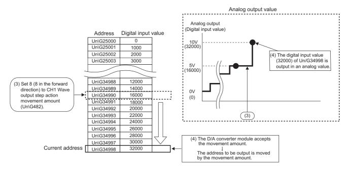
3 Change the digital input value (in the address 34992) to 8000, and set -6 (6 in the reverse direction) to CH1 Wave output step action movement amount (Un\G482).
